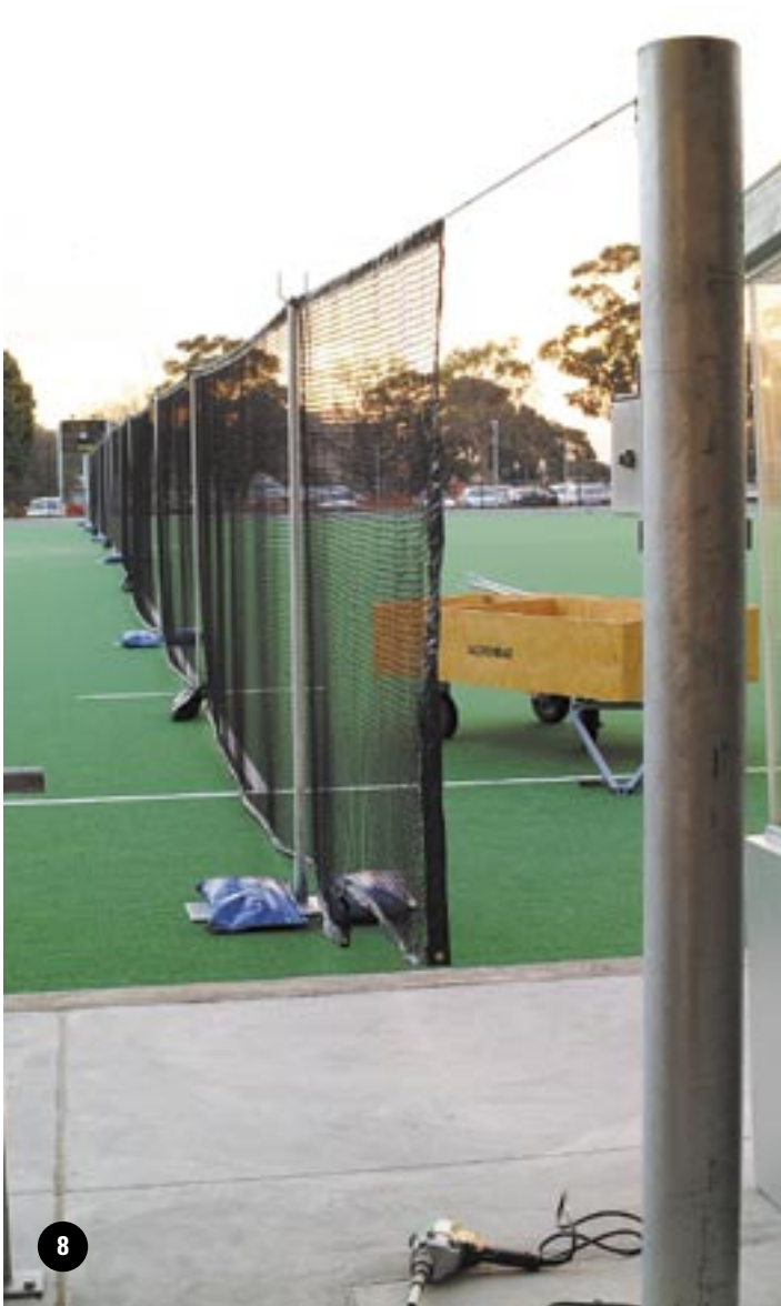
8 A15-113 Dividing Net - Removable, Outdoor, 2400mm High Net: White, 50mm square with black vinyl border, prestretched rope top and weighted bottom. Support posts designed to suit local conditions and intermediate support posts are all included. Finish: Posts - hot dip galvanised. Winch A16-18 and storage box A16-148 ordered separately.
