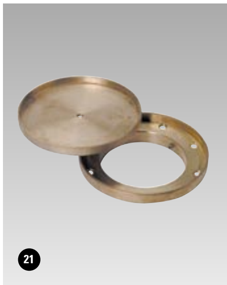
18 A6-43 Cover Plate - Access, 225mm I.D. Use: Large diameter cover for access to power or score board cabling. Cover is reversible. One side is recessed for inlay of flooring. Cover is removed with A6-46 handle. Material: Steel. Finish: Zinc plated. Size: 250mm O.D. x 19mm deep.
