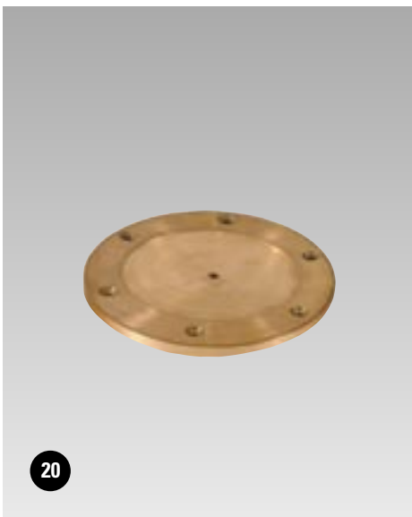
16 A6-44 Cover Plate - Access, 120mm I.D. Use: For access to fixing points and sockets under floors. Cover is reversible. One side is recessed for inlay of flooring material. Cover is removed with A6-46 handle. Material: Steel. Finish: Zinc plated. Size: 145mm O.D. x 19mm deep.
