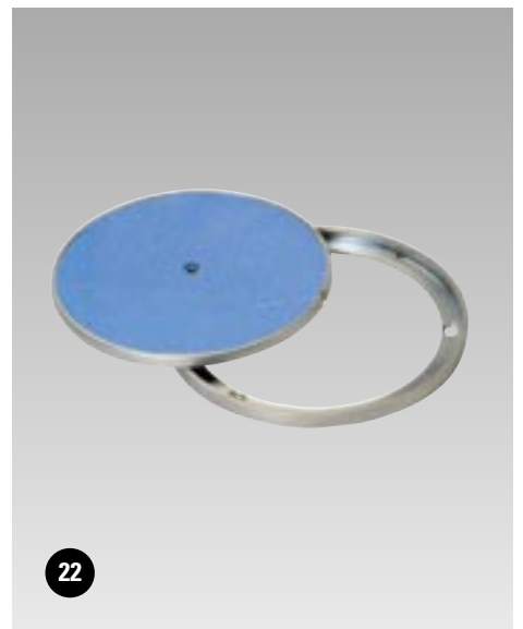
22 A6-48 Cover Plate - Access, 120mm I.D. x 8mm Deep Use: For access to fixing points and sockets under synthetic floors. Low profile for thinner flooring material. Flange has 3 CSK hole for fixing. Cover is reversible. One side is recessed for inlay of flooring material. Cover is removed with A6-46 handle. Material: Steel. Finish: Zinc plated. Size: 145mm O.D. x 8mm deep.
