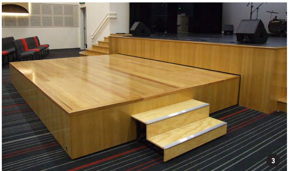
1, 2 and 3 Motorised roll out stage - stored within Height 500mm Timber finish, clear urethane
